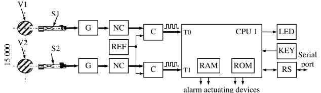
Fig. 1. The block diagram of the measuring channel of the shaft rotational speed
