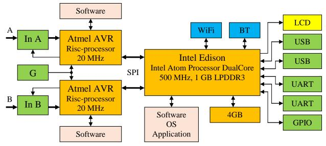
Fig. 1. The block diagram of a microprocessor frequency meter
