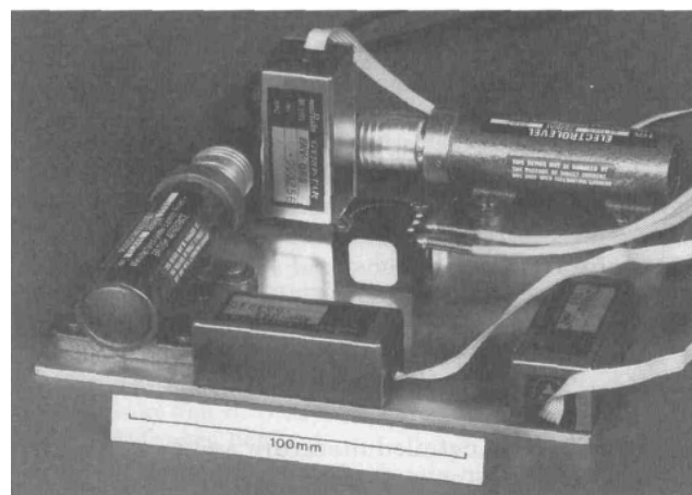
Fig 9. Simply three –axes system for stabilization of the robot platform [3].
