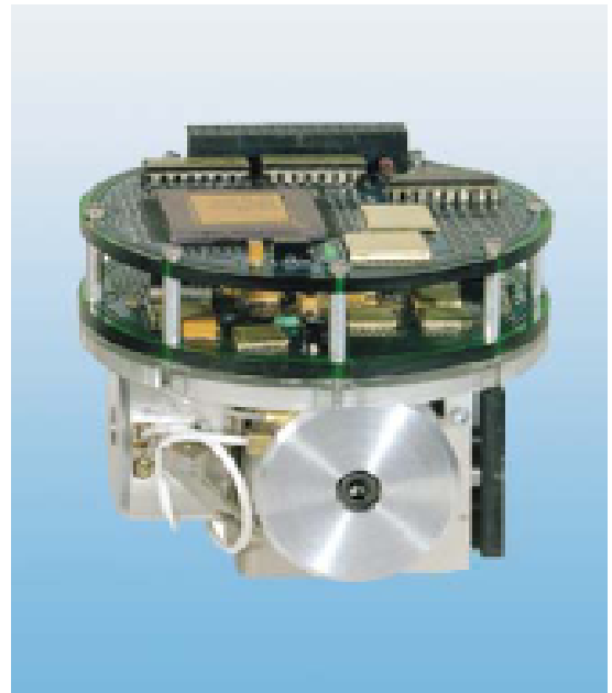
Fig 6 Fiber optic three-axes inertial system LN200 of Northrop Grumman Inc. on the right – without housing
