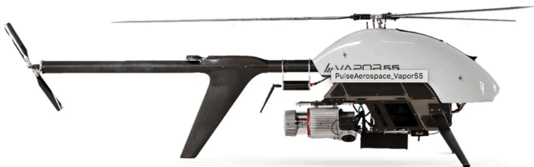
Figure 1.1.3 . single rotor drone
