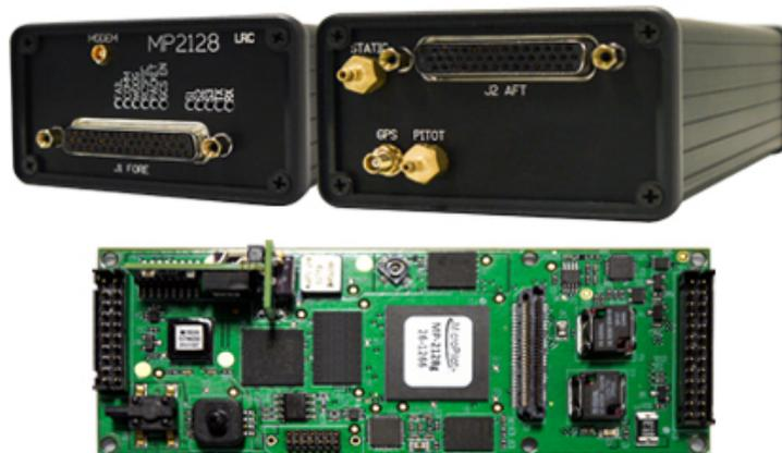
2.3.1.4. MP2128HELI-LRC2 Enclosed helicopter UAV autopilot
