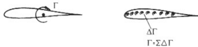
Fig. 12.9 Vortex distribution on the camber line
