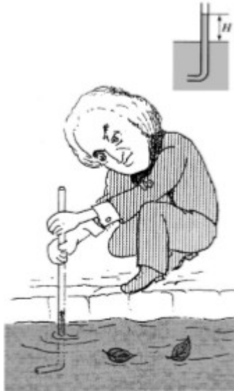
Fig. 7.13 Pitot's first experiment:
