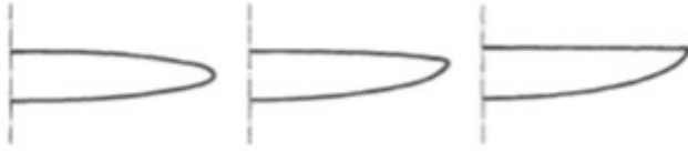
Fig. 16.5 Three different wing planforms with the same elliptic chord distribution
