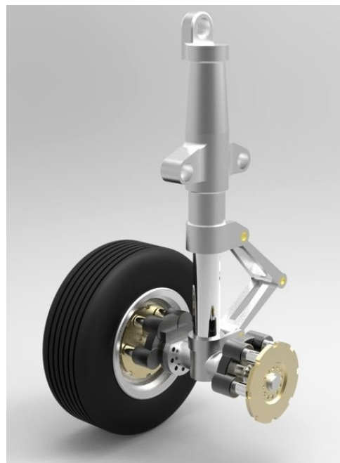
5.3.2 Landing gear main leg with the shock absorber.
