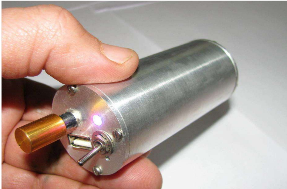
Fig. 23 The ultrasonic portable leak tester “Koloran”
