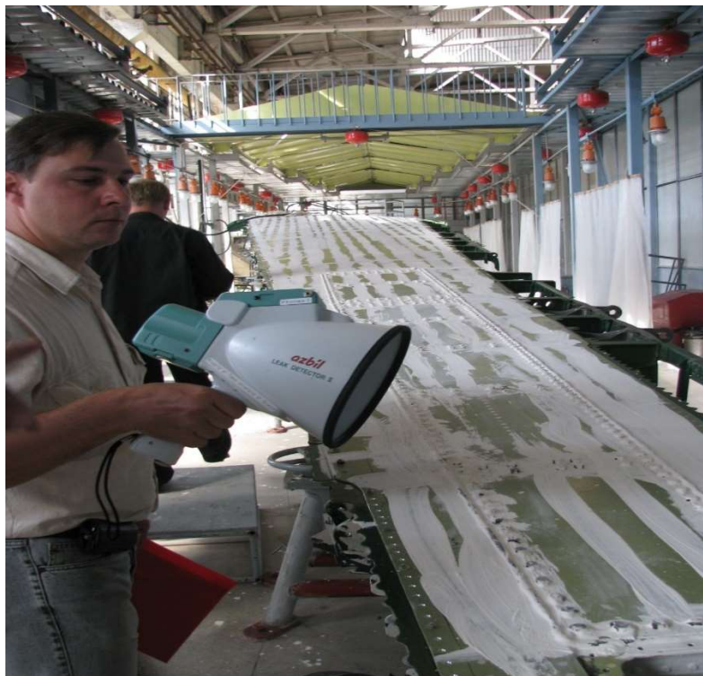
Fig. 24 Testing of throws defects in fuel tanks of AN-148 plane. It shows using of the capillary kerosine-chalk method and ultrasonic leak testing (the detector “AZBIL”) of the plane’s wing rivets.
