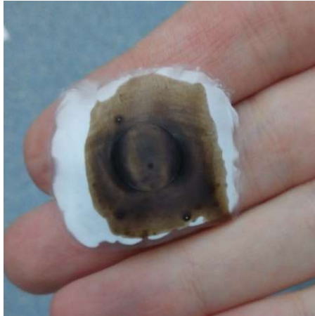
Fig. 17 - Replica obtained using fluorovinyl-fluoropropylene copolymer.
