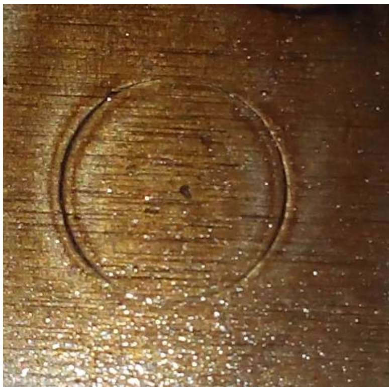
Fig. 18 - Defect image obtained by method 3, using fluorovinyl-fluoropropylene copolymer and CM with a concentration of 0.8 g/l.
