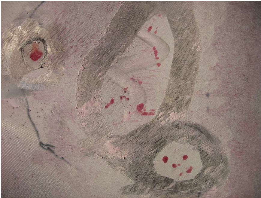
Fig. 8 Dye "traces" of defects on the test surface of the fuel tank
