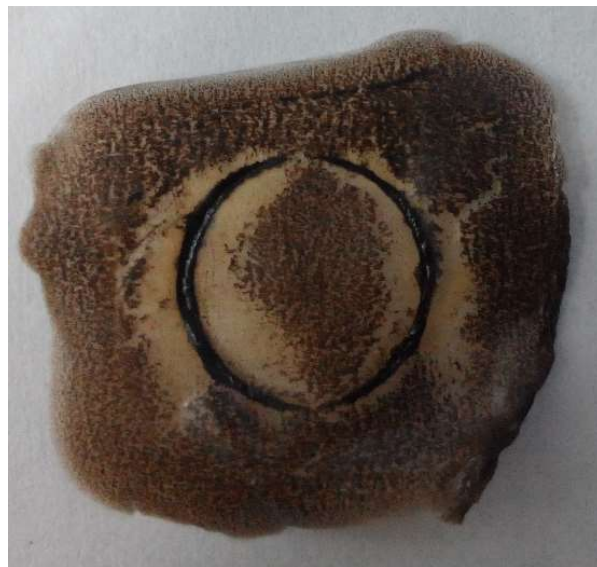
Fig. 16 - Replica formed by composition with polyvinyl acetate.
