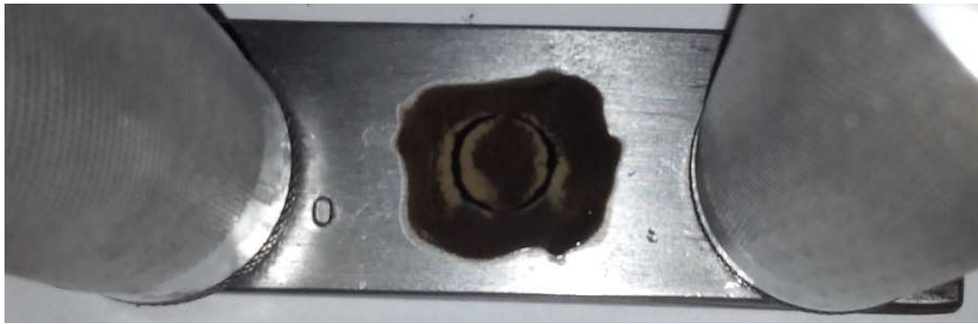
Fig. 15 - Formation of an image of a defect by composition with polyvinyl acetate.
