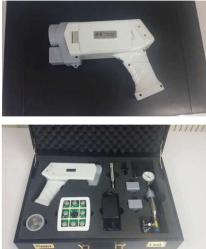
Fig. 28 Picture of the portable ultrasonic leak detector
