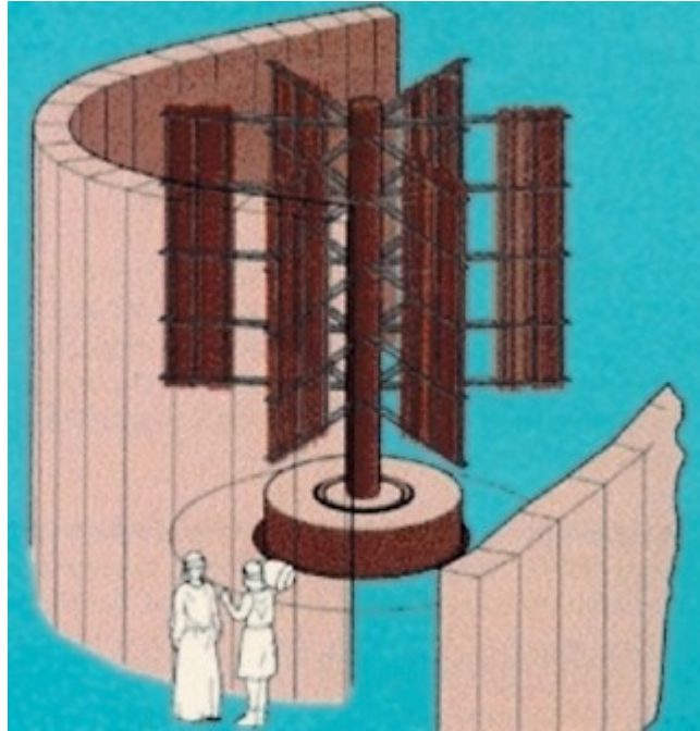
Figure 13 Ancient Persian mill with a wind guide Wall
