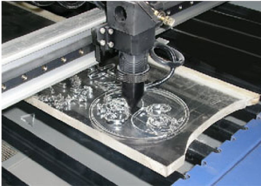
Figure 55 Laser cutting of plastic
